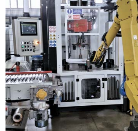
ELECTRIC PRESS MACHINES FROM 15 TO 100 TON FOR INSERTING SHAFT COLD - HOT PROCESS
